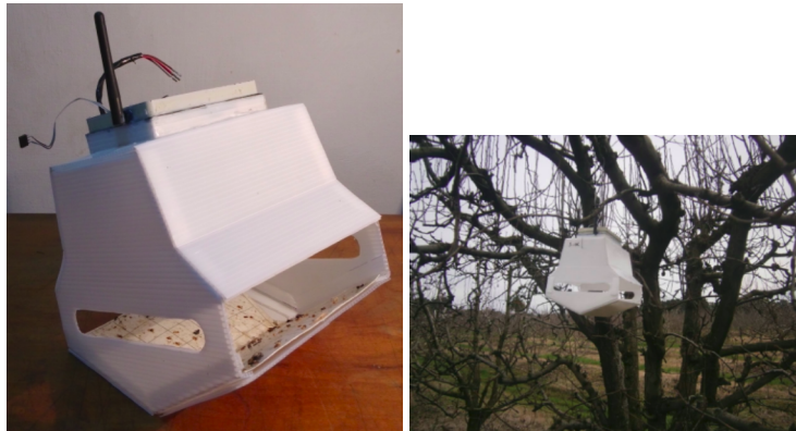
Figure 2: The system for insect monitoring and early warning for plague prevention.
